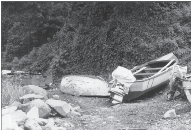
Figure 3. The “double ender” (centre) and “bow and stern” (right) typically used by fishermen on the west coast of St. Vincent for the capture of flyingfish.
