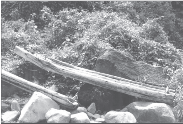
Figure 1. The “logwood” or catamaran typically used by fishermen on the north and northeast coasts of St. Vincent for the capture of flyingfish.
