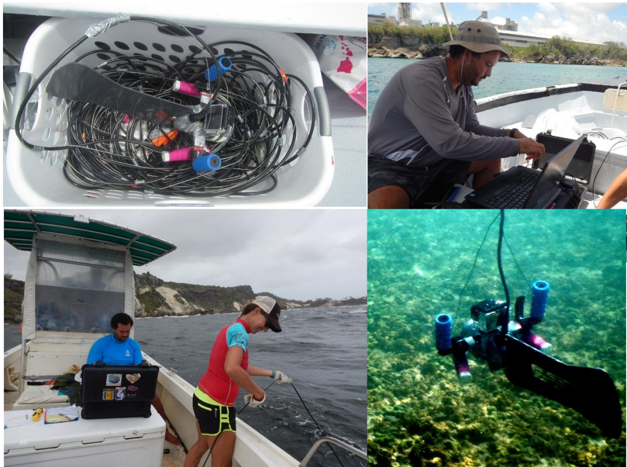
Figure 5. Photographs showing the setup and operation of equipment at the field sites. Top left: camera rigging and cable stored in a basket between sites; top right: dell latitude laptop resting on the pelican case; bottom left: deployment and monitoring of camera equipment over the side of the vessel; bottom right: camera equipment recording videos approximately 1 m above the substrate.
