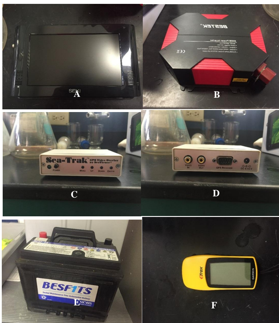
Figure 6. Photographs of some of the equipment used in the SeaViewer setup; A - seiki portable screen; B - Bestek power inverter; C - SeaTrak gps video overlay receiver (front view); D - SeaTrak gps video overlay receiver (rear view); E - Besfits 12v marine battery; F - Garmin e-Trex handheld gps.
