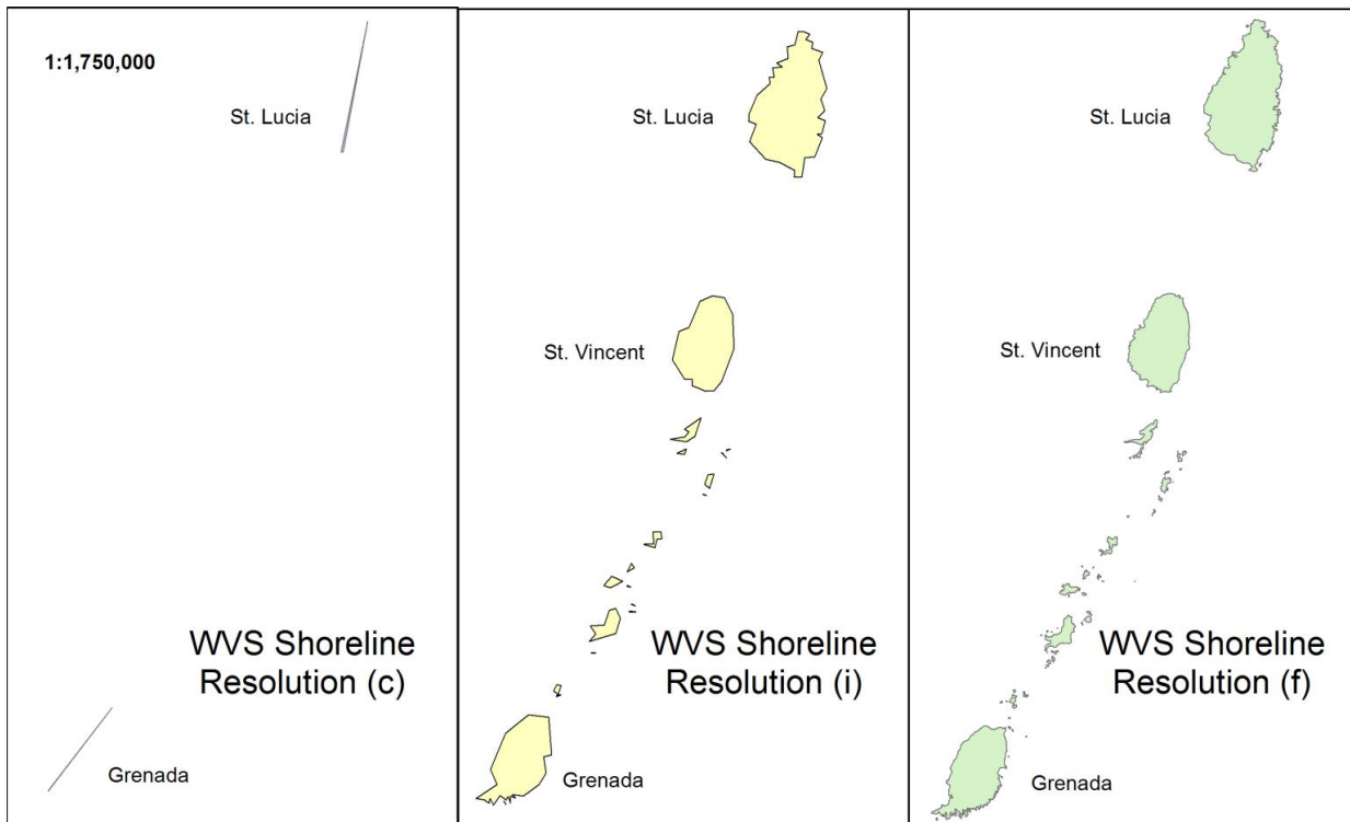
Figure 1. Map of selected Eastern Caribbean countries to show the accuracy between the various levels of shoreline resolution provided by the WVS dataset.
